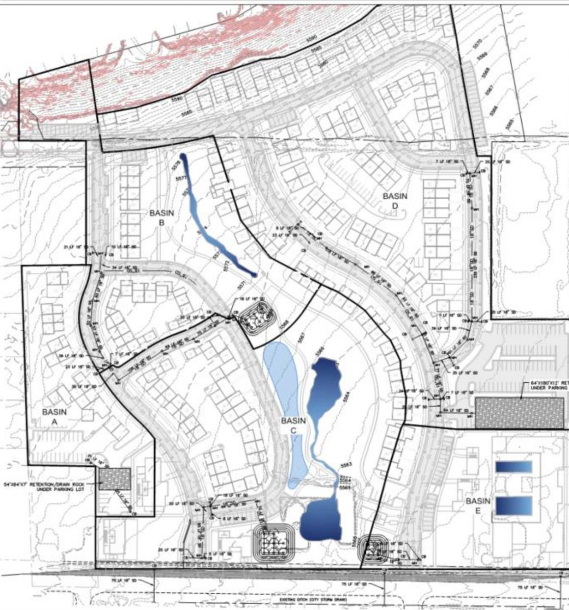
Test pits in the project report generally show depths under 1' of basins. Assume penetration of 2.0 inches per foot for all pits. Drainage areas to the northwest ending at 15' of slope. Retention area under the parking lot is 1.0 acre.
